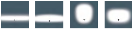
[P65] Pedestrian/bicycle lane [S70] Streetlighting [A60] Asymmetric 'forward throw' [R65] Rectangular 'forward throw'
