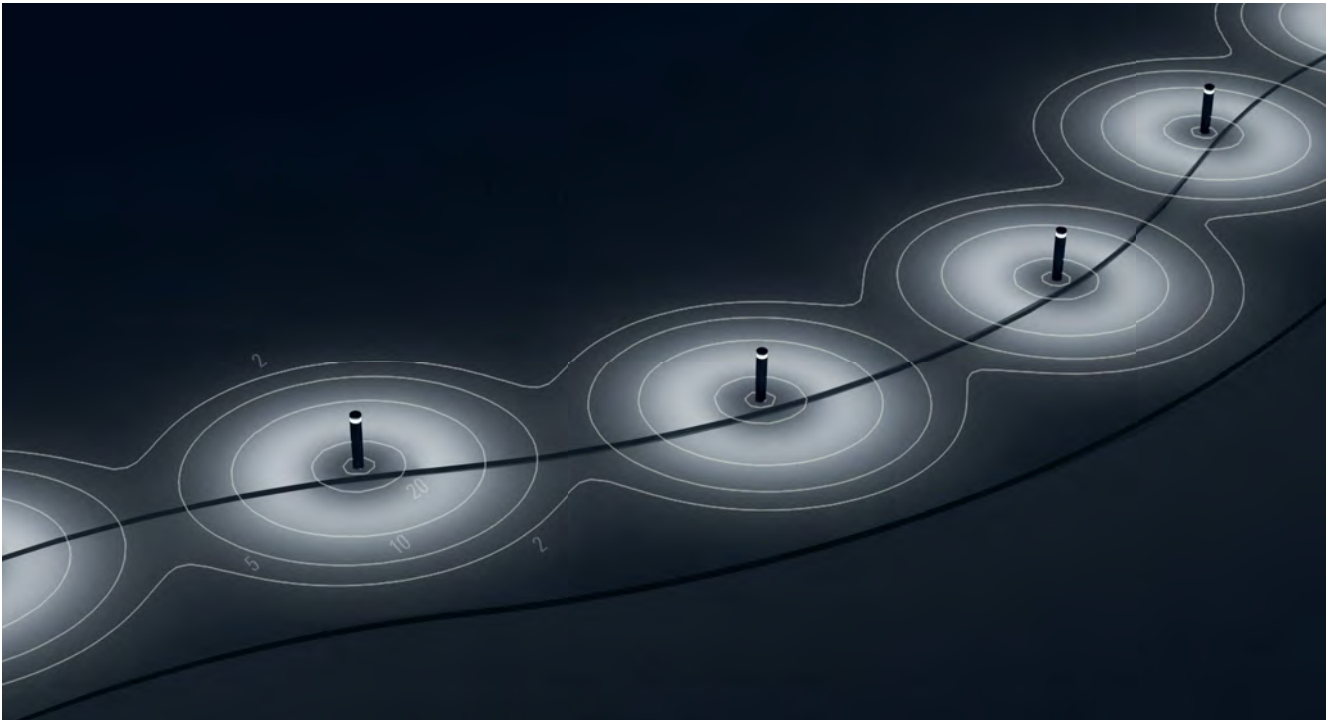
ZFY230 [C60] 12 W 4000 K LLF = 0.9 Luminaire spacing 7.0 metres Path width 4.0 metres
