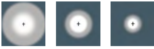
[B] Symmetric, wide beam [M] Symmetric, medium beam [EE] Symmetric, very narrow beam
