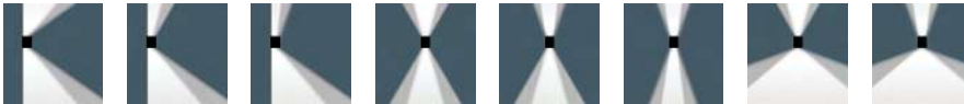
[R45/R45] 'Side throw', up and down [M/R45] Medium beam up, 'side throw' down [E/R45] Narrow beam up, 'side throw' down [M/M] Medium beam, up and down [E/M] Narrow beam up, medium beam down [E/E] Narrow beam, up and down [M/S] Medium beam up, 'side throw' down [E/S] Narrow beam up, 'side throw' down
