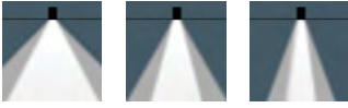
[B] Symmetric, wide beam [M] Symmetric, medium beam [E] Symmetric, narrow beam
