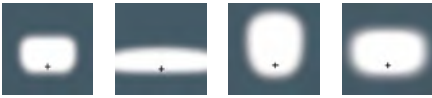
[R45] Rectangular 'side throw' [S70] Asymmetric 'side throw' [A60] Asymmetric 'forward throw' [R65] Rectangular 'side throw'
