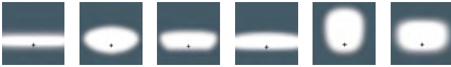
[P65] Pedestrian/bicycle lane [S60] [S65] [S70] Streetlighting [A60] Asymmetric 'forward throw' [R65] Rectangular 'side throw'
