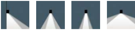
[R45] Rectangular 'side throw' [M] Symmetric, medium beam [E] Symmetric, narrow beam [S] Asymmetric 'side throw'
