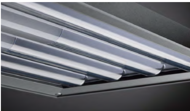
The contour of the main lens follows the shape of the individual LED lens, thereby minimising internal reflections within the luminaire.
